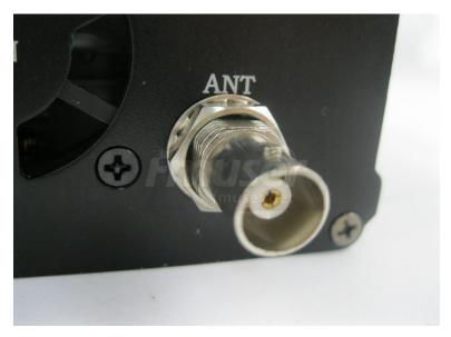
In the back of the transmitter, the antenna interface (ANT) as a BNC interface, therefore, the antenna interface should also be as BNC. External power adapter output
